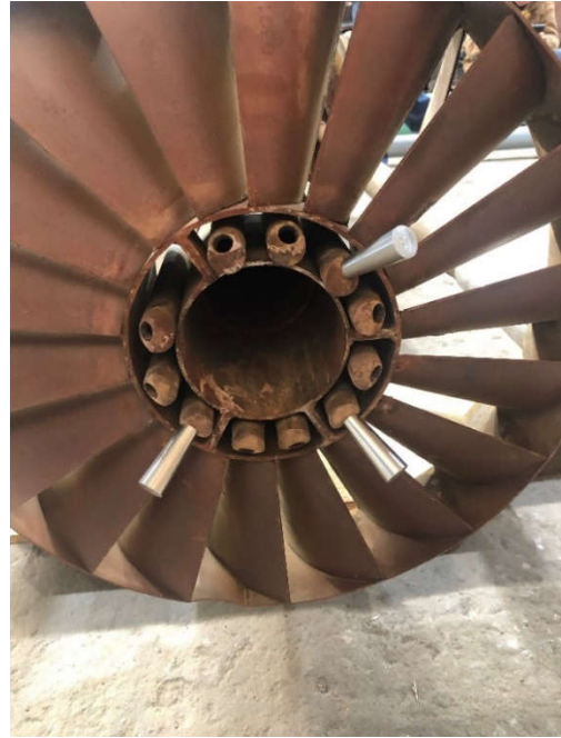
Figure 1: Taper Pins Installed
