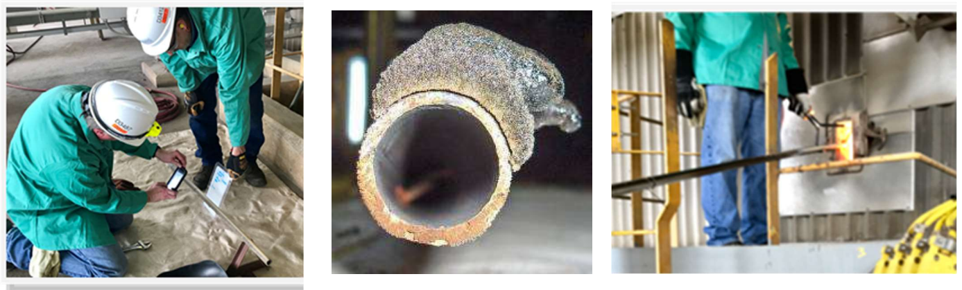
Figure 3. A high temperature probe duplicates generating tube surface temperatures to simulate deposit bond and deposition rate. Deposits are then collected and analyzed by a third-party laboratory. The tests are repeated to optimize reagent type and dosage.
