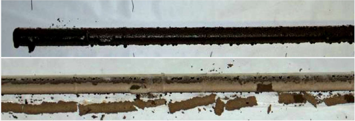
Figure 4. The baseline high temperature probe (HTP) testing at a PRB-fired 640MW opposed wall furnace produced a heavy layer of black glass that adhered to the probe (top). The coal was pretreated with CT-300 at an initial "shock" dosage and later optimized to a reduced maintenance dosage. HTP testing was repeated one day later and the coating on the probe was more porous, friable, and cracked off as it was removed from the inspection port (bottom), confirming the sticky alkali layer of slag was prevented from forming.
